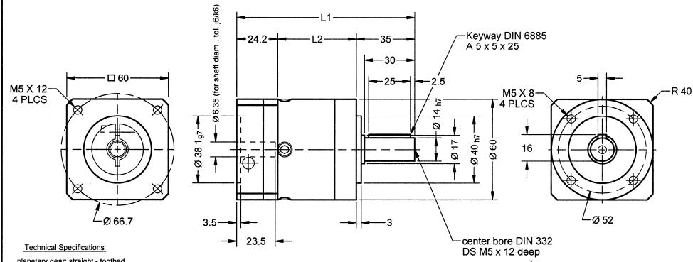
planetary gear: straight - toothed output shaft bearing: grooved ballbearing
